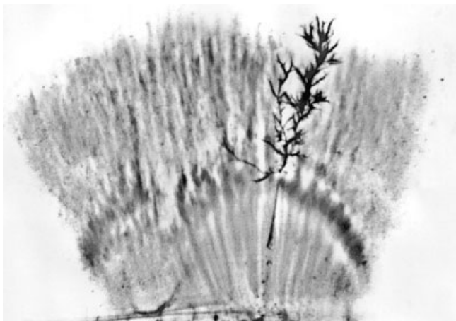
Figure 5 Electrical tree grown inside a water tree in laboratory conditions.
